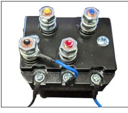
Connect BLUE post to the winch BLUE post Connect YELLOW post to the winch YELLOW post Connect RED post to the battery POSITIVE post Connect BLACK post to the battery NEGATIVE post
